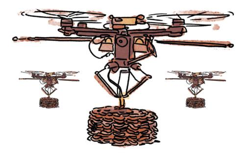
AAM uses fleets of drones working together from a single blueprint to 3D-print structures, depositing materials during flight to build from the air.
