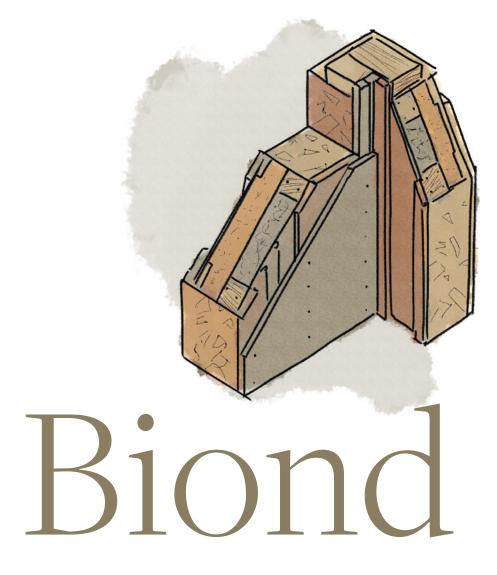
A closed timber frame panel construction system, insulated with a mix of wood fibre, hemp and lime. Created by Greencore Homes to build its 'climate positive homes', it is better than net zero in terms of embodied carbon, with no offsetting required.
