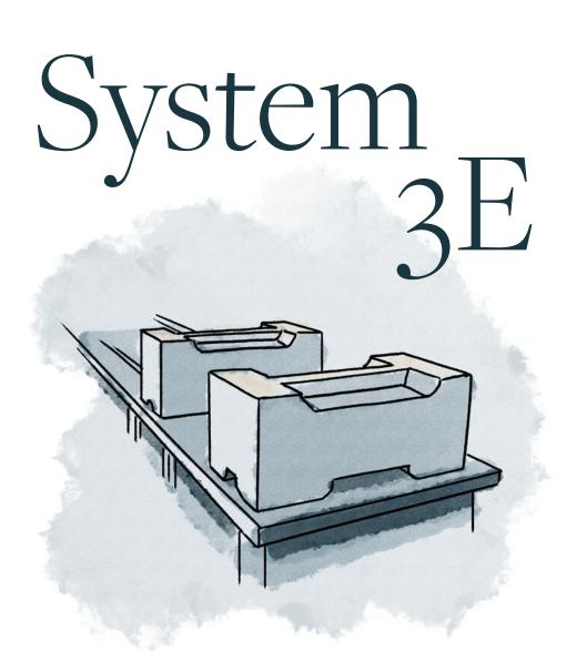
LEGO®-like building blocks that fit together tightly without mortar, and contain expanded perlite, a naturally occurring volcanic glass that is highly insulating.
