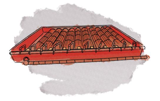
A solar-powered, natural algae-fuelled system that automatically cleans waste water and provides fresh water for construction and agricultural uses in local communities affected by water shortages.
