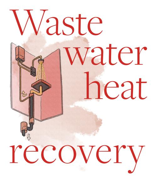
A process that recovers heat from hot water that would normally go down the drain and uses it to preheat cold water. It is a sustainable and cost-effective way to reduce energy consumption and carbon emissions in buildings.
