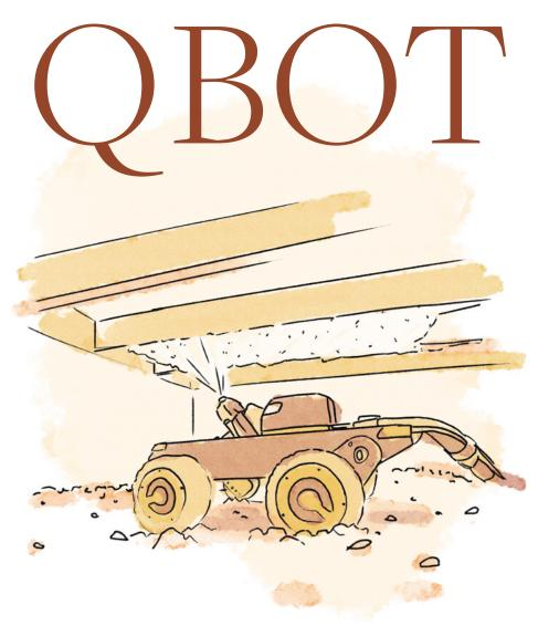
A robot that can crawl through tight spaces under floors and install insulation in older homes without requiring major renovations, helping to improve energy efficiency and reduce carbon emissions.
